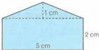
$$\left. \begin{aligned} A_1 &= b \cdot h = 5 \cdot 2 = 10 \text{ cm}^2 \\ A_2 &= \frac{b \cdot h}{2} = \frac{5 \cdot 1}{2} = 2,5 \text{ cm}^2 \end{aligned} \right\} \rightarrow A = A_1 + A_2 = 10 + 2,5 = 12,5 \text{ cm}^2$$
